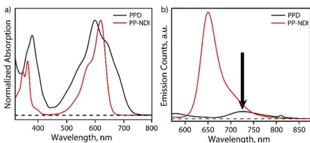
Fig. 2 (a) Steady state absorption spectra of PPD (in black) and PP-NDI (in red) in DCM at 200  $\mu\text{M}$  concentration, respectively. The PPD spectrum shows clear evidence of strong electronic coupling between the NDI scaffolds. (b) Steady state emission spectra of PPD (black) and PP-NDI (red) in DCM at 200  $\mu\text{M}$  concentration, subsequent to excitation at 540 nm.
