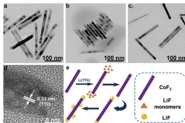
Fig. 3 TEM images of samples after 9 months: (a)  $\text{CoF}_2$ - $\text{LiF}$  heterostructures (0.05 mmol), (b)  $\text{CoF}_2$  nanorods, (c)  $\text{CoF}_2$ - $\text{LiF}$  heterostructures (0.01 mmol), (d) HR-TEM image of  $\text{CoF}_2$ - $\text{LiF}$  heterostructures (0.05 mmol), and (e) schematic of the formation of  $\text{CoF}_2$ - $\text{LiF}$  heterostructures.
