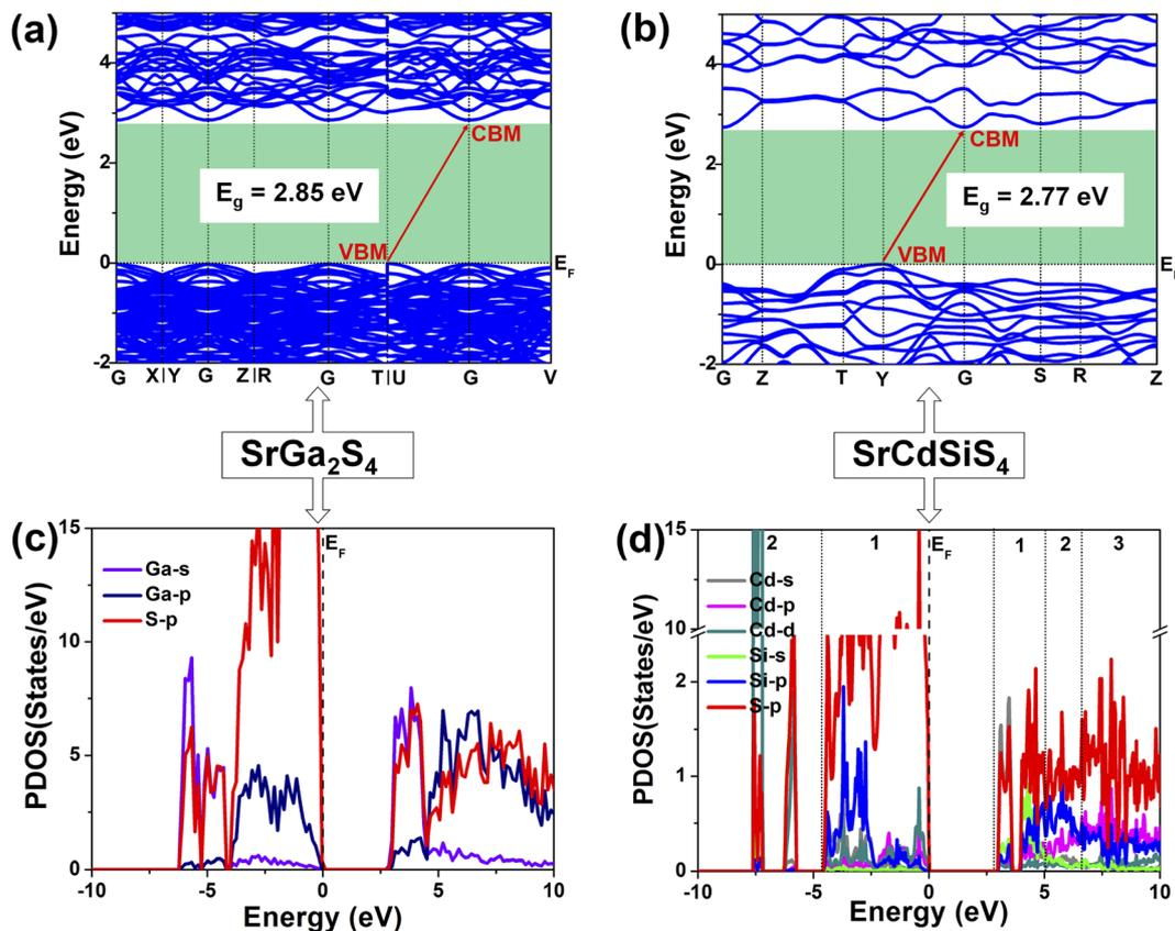
Fig. 5 Changes in (a and b) electronic band structures and (c and d) PDOSs (states with less contributions are omitted for better view) from SrGa<sub>2</sub>S<sub>4</sub> to SrCdSiS<sub>4</sub> caused by dual-site aliovalent substitution.
