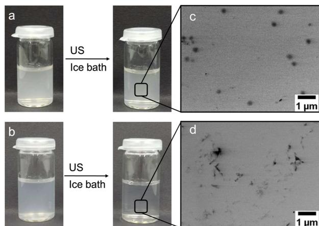
**Fig. 2** Photographs before and after 10 min ultrasonication at 30% amplitude and 20 kHz in an ice bath of (a) B1.5 and (b) Se1.5 microgels. STEM images of (c) B1.5 and (d) Se1.5 microgels after ultrasonication.
