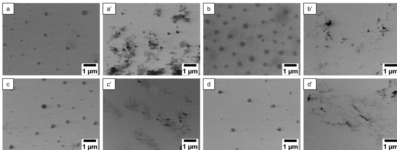
Fig. 4 STEM images of  $\text{Se}_{1\mu}\text{G}$  before sonication of (a) 0.5, (b) 1.5, (c) 3.0, and (d) 5.0 mol% diselenide content. The images after 10 min sonication (a'), (b'), (c'), and (d') correspond to (a), (b), (c), and (d), respectively. Sonication was carried out in an ice bath at 30% amplitude for 10 min.
