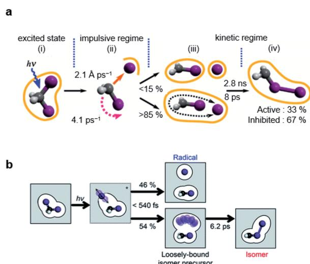
Fig. 5 Photochemical dynamics of  $\text{CH}_2\text{I}_2$  in (a) cyclohexane and (b) methanol, from fs-TRXL studies. The scheme in (a) is reproduced from ref. 66 with the permission of the American Physical Society, copyright 2020, and the scheme in (b) is reproduced from ref. 67, with the permission of the Royal Society of Chemistry, copyright 2021.
