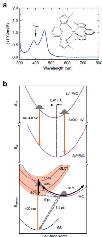
Fig. 8 (a) UV-visible absorption spectrum of  $[\text{Fe}(\text{bmip})_2]^{2+}$  in acetonitrile with its chemical structure (inset). (b) Schematic representation of the excited-state dynamics of  $[\text{Fe}(\text{bmip})_2]^{2+}$  determined from a combined study of TR-XES and fs-TRXL. Reproduced from ref. 70 with the permission of Springer Nature, copyright 2020.
