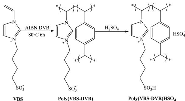
Scheme 1 Synthesis of acidic polymeric ionic liquids.
