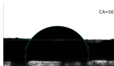
Fig. 3 The contact angle of water on the surface of Poly(VBS-DVB)HSO<sub>4</sub>.
