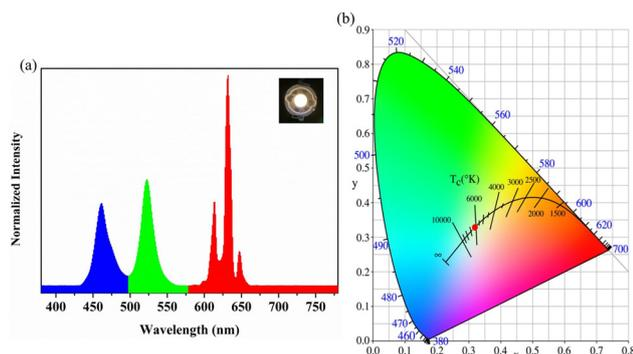
**Fig. 8** (a) PL emission spectrum. The inset shows the photograph of device in open states; (b) CIE coordinates of NADES-CsPbBr<sub>3</sub> PNCs in CIE space.
