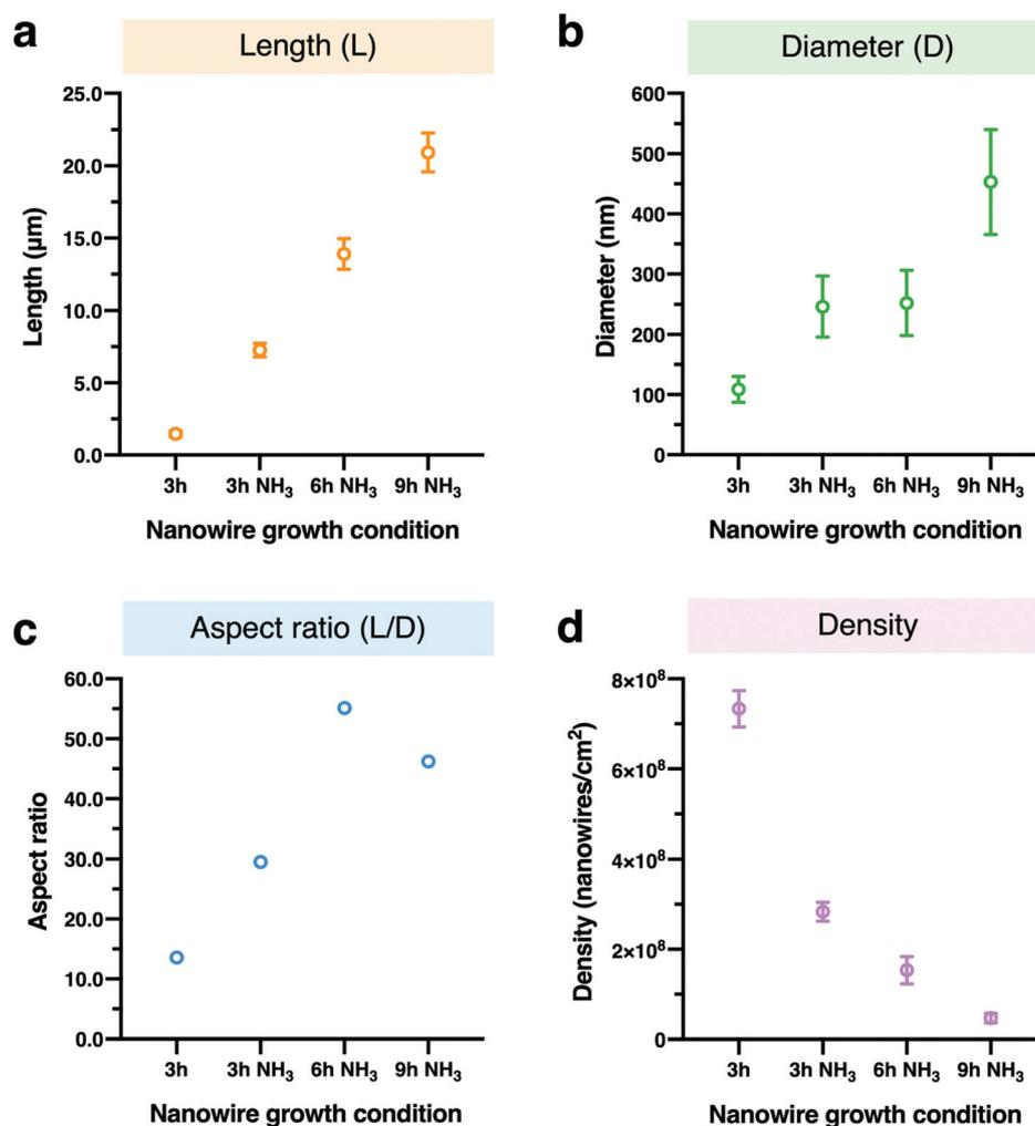
**Fig. 2** The dependence of the morphology of ZnO nanowires on four nanowire characteristics. (a) Statistic length and (b) diameter of nanowires. The error bars are defined by standard deviation values ( $n = 100$ ). (c) Aspect ratio (length/diameter) of nanowires. (d) Density of nanowires calculated by counting the tips of nanowires in a known area. The error bars are defined by standard deviation values ( $n = 490, 190, 100, 30$  counted nanowires at each condition, respectively).
