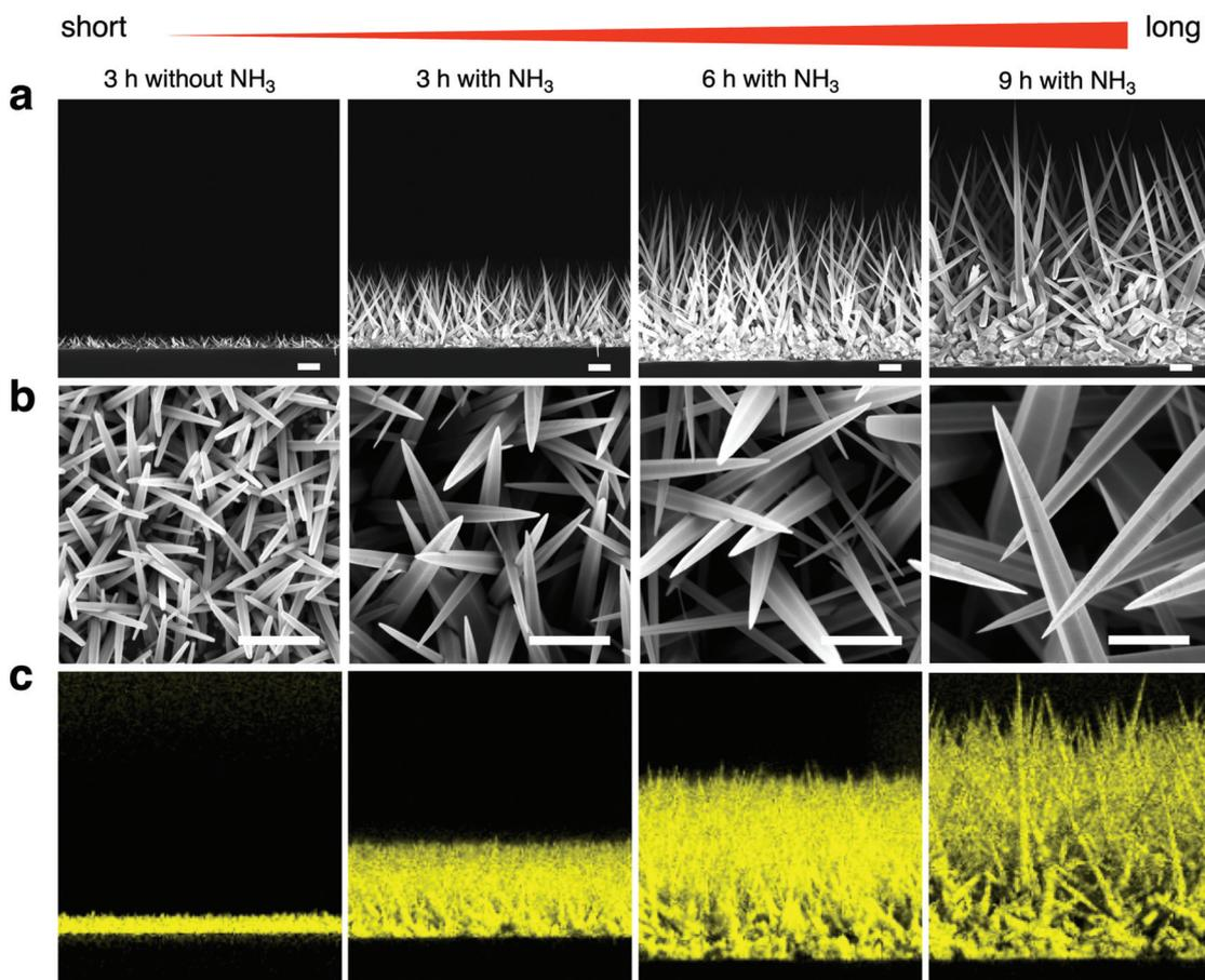
**Fig. 1** (a) FESEM images of cross-sectional nanowires for different growth conditions. The scale bars are 2  $\mu$ m. (b) FESEM images of top-view nanowires. The scale bars are 1  $\mu$ m. (c) Elemental mapping of Zn K $\alpha$  (8.6313 keV) highlighted in yellow, as a main constituent of the nanowires.
