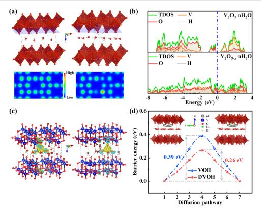
Fig. 4 (a) Optimized crystal structure of VOH and DVOH and corresponding charge distribution sliced along the (00I) direction. (b) Calculated DOS of the VOH and DVOH. (c) Charge density difference of the Zn/VOH and Zn/DVOH (yellow areas: electron depletion. Light blue areas: electron accumulation). The isosurface is set to be 0.005 e  $Å^{-3}$ . (d) Diffusion barrier profiles of  $Zn^{2+}$  transport in DVOH and VOH nanosheets along the b axis (insets show the Zn<sup>2+</sup> diffusion process).
