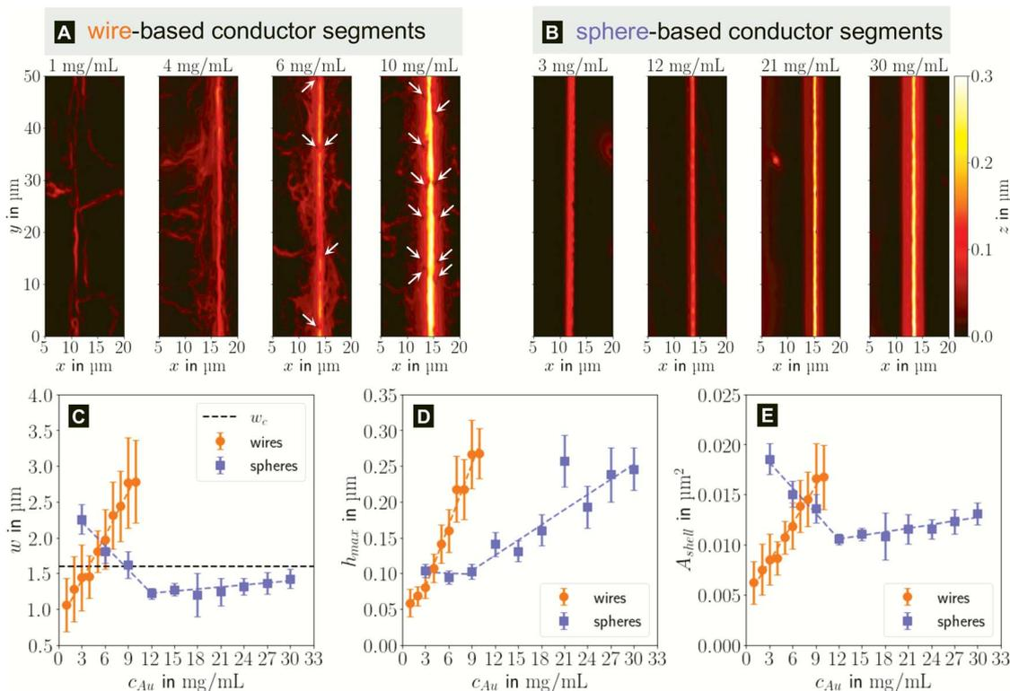
Fig. 4 Topography maps of (A) wire- and (B) sphere-based printed lines after plasma sintering. White arrows indicate defects similar to those in Fig. 2C. (C) Average conductor width  $w$ , (D) maximum conductor height  $h_{\text{max}}$  and (E) cross-sectional area  $A_{\text{shell}}$  as a function of gold concentration  $c_{\text{Au}}$ . Standard deviations are indicated as error bars, the dashed lines are fits by linear regression to better illustrate the (piece-wise) linear behaviour.
