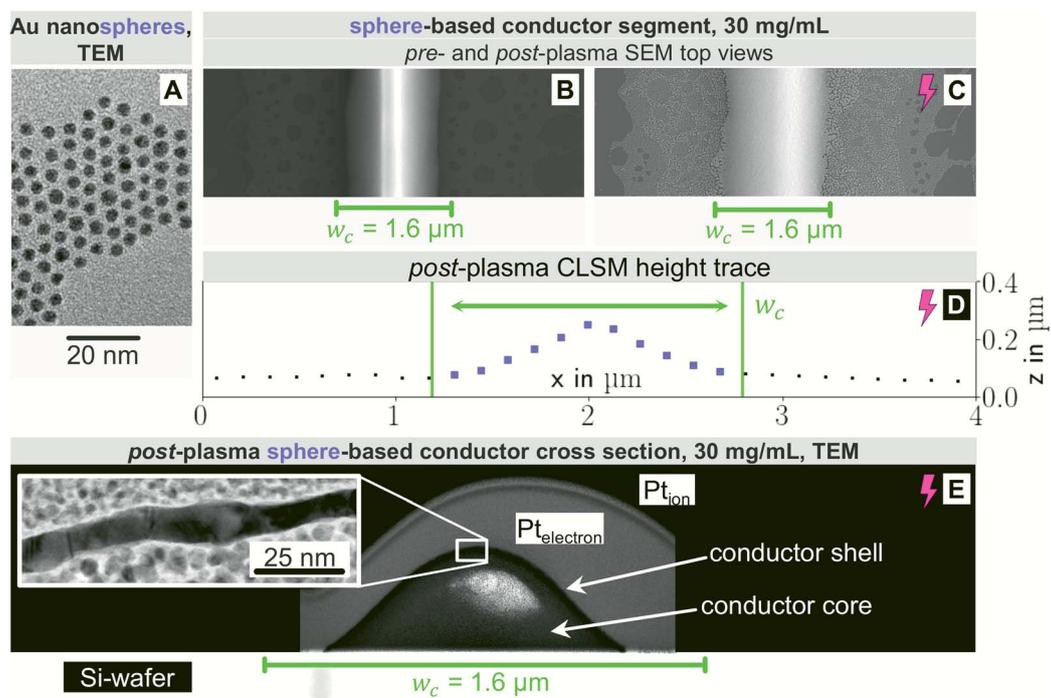
Fig. 3 Typical morphological features of lines printed from AuNP at  $c_{Au} = 30 \text{ mg mL}^{-1}$  before and (purple flash) after plasma. (A): TEM image of dried and self-assembled spheres. (B): SEM image (top-view) of a printed line. (C): SEM image (top-view) of a printed, plasma-sintered line. (D): Height trace of a printed, plasma-sintered line. (E): TEM image of a cross-section of a printed, plasma-sintered line. Inset: A shell formed by the plasma.
