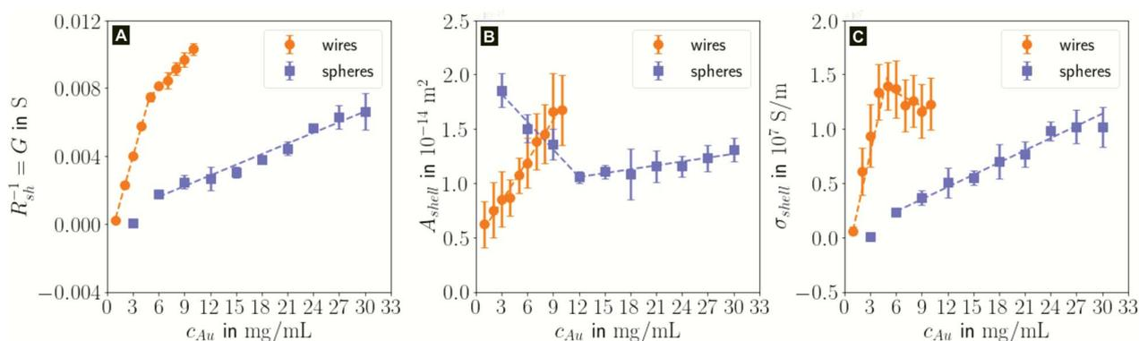
Fig. 5 Effect of particle concentration  $c_{\text{Au}}$  on (A) the conductance  $G$  of a representative square electrode sub-section, (B) the cross-sectional area  $A_{\text{shell}}$  and (C), the shell conductivity  $\sigma_{\text{shell}}$ . Standard deviations are indicated as error bars, the dashed lines are fits by linear regression to better illustrate the piece-wise linear relations.
