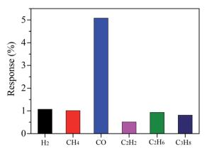
Fig. 11 Selectivity of the Ag-ZnO-MoS<sub>2</sub> nanocomposite sensor towards 100 ppm gas species of H<sub>2</sub>, CH<sub>4</sub>, CO, C<sub>2</sub>H<sub>2</sub>, C<sub>2</sub>H<sub>6</sub> and C<sub>3</sub>H<sub>8</sub> (reproduced from ref. 143 with permission from Elsevier).
