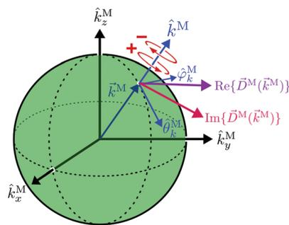
Fig. 3 Sketch of the (complex) photoionization dipole  $\vec{D}^M(\vec{k}^M) \equiv \langle \hat{k}^M | \vec{d} | 0 \rangle$  for a particular value of the photoelectron momentum  $\vec{k}^M$ . Red circular arrows indicate the direction of left (+) and right (−) circular polarization with respect to  $\vec{k}^M$ .
