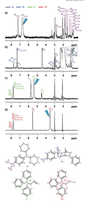
Fig. 4 Multiplet selective excitation 1D  $^1$ H NOESY spectra of a phosphorus-based compound test mixture (20 mM) dissolved in sulfolane/DMSO-d<sub>6</sub> (7:3 v/v) (a–d),  $t_{\rm m}$  = 1 s, at 258 K, at 500 MHz ( $^1$ H). The initial selective inversion pulses excite: (a) H<sub>16,18</sub>(1a), (b) H<sub>2a</sub>(1b), (c) H<sub>10</sub>(1c), and (d) H<sub>10</sub>(1d) proton resonances. Reproduced with permission from ref. 69, © 2020 American Chemical Society.
