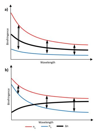
Fig. 2 Graphical representation of (a)  $n_0$  is smaller and less wavelength dependant giving positive dispersion and (b) when  $n_0$  is larger and more wavelength dependant giving negative dispersion.
