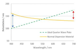
Fig. 1 Retardation profiles for an ideal quarter-wave plate and material with normal dispersion optimised for a wavelength of 550 nm. Arrows denote the discrepancy observed at different wavelengths.
