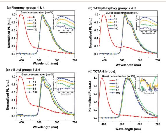
Fig. 2 PL spectra of neat and blend films of 1 and 4 (a), 2 and 5 (b), 3 and 6 (c) and TCTA and Ir(ppy)<sub>3</sub> (d) at different concentrations excited at 330 nm. The PL data of neat Ir(ppy)3 was taken from the literature. 23 Inset figures show the PL spectra at shorter wavelengths with the PL intensity on a logarithmic scale.
