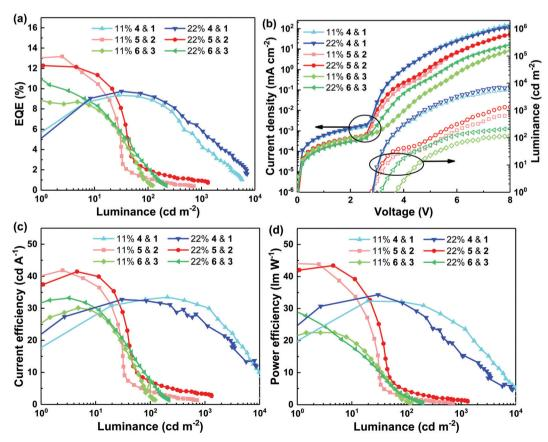
Fig. 5 EQE (a), CE (c) and PE (d) versus luminance and J-V-L characteristics (b) of OLEDs composed of different material combinations at different ratios
