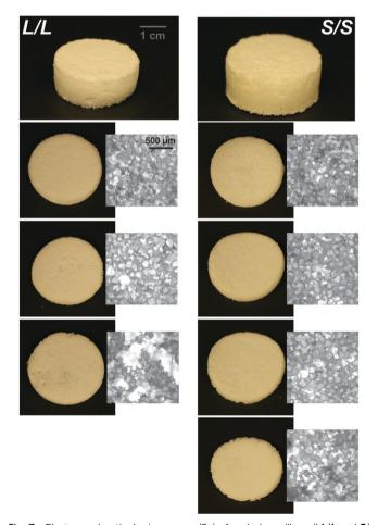
Fig. 7 Photos and optical microscopy (5x) of scaled-up, "large" L/L and S/S scaffolds ( $d\sim24$  mm) demonstrating superior macromer diffusion, and more uniform pores, for the S/S composition.
