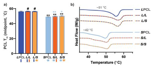
Fig. 2 (a) Midpoint tm of PCL of scaffolds; \*p < 0.05, \*\*p < 0.01, #p > 0.05. Note: the black color-coded statistics are comparisons to *LPCL* and blue color-coded statistics are comparisons to SPCL. (b) Representative thermogram for each scaffold composition.
