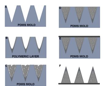
Fig. 5 (A) PDMS mold. (B) Deposition of polymeric solution on PDMS mold. (C) Dried layer. (D) MNs filled with MPs. (E) Compacted and HL applied. (F) MNs extracted from mold. MPs, which are pressed and plasticized by using a non-invasive soft plasticization method previously reported.19
