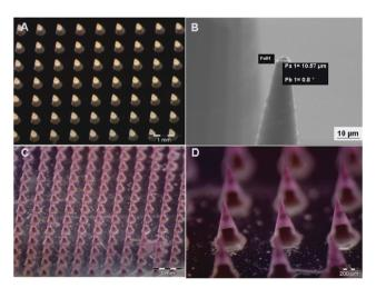
Fig. 6 (A) Stereomicroscope micrographs of master fabricated using 2-photon polymerization. (B) SEM micrograph of the master tip. (C and D) Stereomicroscope micrographs of microneedle patches with rhodamineloaded tips.
