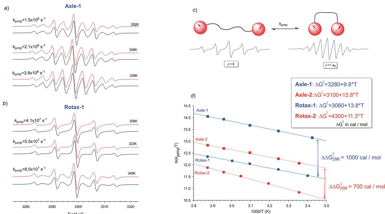
Fig. 2 EPR spectra of **Axle-1** (a) and **Rotax-1** (b) recorded in MeCN at various temperatures. In black are reported the corresponding theoretical simulations obtained by using the rates of exchange reported in the figure and by assuming a two-state jump model (c) where  $k_{\text{jump}}$  represents the apparent rate of jumping between two set of conformations having and  $J = 0$  and  $J \gg a_N$ . (d) Plots of  $\ln(k_{\text{jump}}/T)$  versus  $1000/T$  for the different biradicals.
