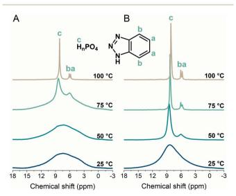
Fig. 3 Variable-temperature <sup>1</sup>H magic-angle spinning (MAS) solidstate NMR spectra (MAS 8 kHz) of (A) 1 and (B) 1g from 25 to 100 °C.
