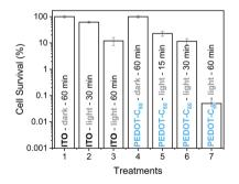
Fig. 10 Survival of *S. aureus* biofilm on ITO electrode (treatments 1–3) and on PEDOT- $C_{60}$  (treatments 4–7). (1) Control: biofilm on ITO electrode kept in dark 60 min. (2) Control: biofilm on ITO electrode irradiated 30 min. (3) Control: biofilm on ITO electrode irradiated 60 min. (4) Control: biofilm on PEDOT- $C_{60}$  kept in dark 60 min. (5) Biofilm on PEDOT- $C_{60}$  irradiated 30 min. (7) Biofilm on PEDOT- $C_{60}$  irradiated 60 min. Samples were irradiated with visible light.
