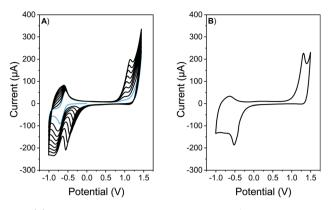
Fig. 1 (A) Repetitive cyclic voltammograms of a 0.5 mM solution of EDOT- $C_{60}$  in TBAPF<sub>6</sub> (0.1 M)/DCM. Light blue line denotes the first cyclic voltammogram. (B) Cyclic voltammogram of a PEDOT- $C_{60}$  film electro-deposited on ITO electrode in TBAPF<sub>6</sub> (0.1 M)/DCM. Scan rate: 50 mV s<sup>-1</sup>.
