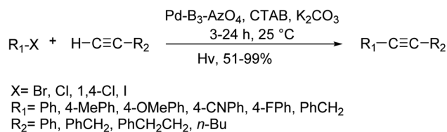
Scheme 61 The Sonogashira reaction in the presence of the Pd-B 3 -AzO 4 .
