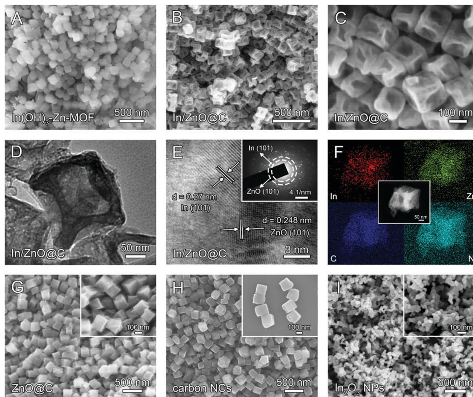
Fig. 1 SEM images of (A) In(OH)<sub>3</sub>-Zn-MOF precursors and (B and C) In/ZnO@C. (D) TEM, (E) HRTEM (inset, SAED pattern), and (F) elemental mapping images of In/ZnO@C. SEM images of (G) ZnO@C, (H) carbon NCs and (I) In<sub>2</sub>O<sub>3</sub> NPs.
