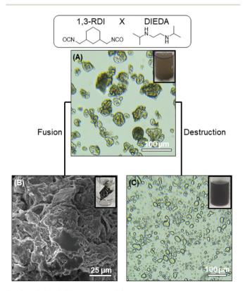
Fig. 2 1,3-RDI-DIEDA capsules: (A) optical microscopy image of capsules dispersed in dodecane; (B) SEM image of monolith after capsule fusion; (C) optical microscopy image of droplets after capsule destruction by hexylamine. Inset images are photographs of the samples.
