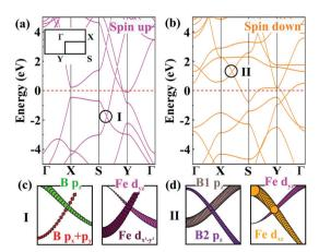
Fig. 4 Band structures of the  $\alpha$ -FeB<sub>3</sub> monolayer for the (a) spin up and (b) spin down channels. The orbital-resolved band structures of Dirac point (c)
