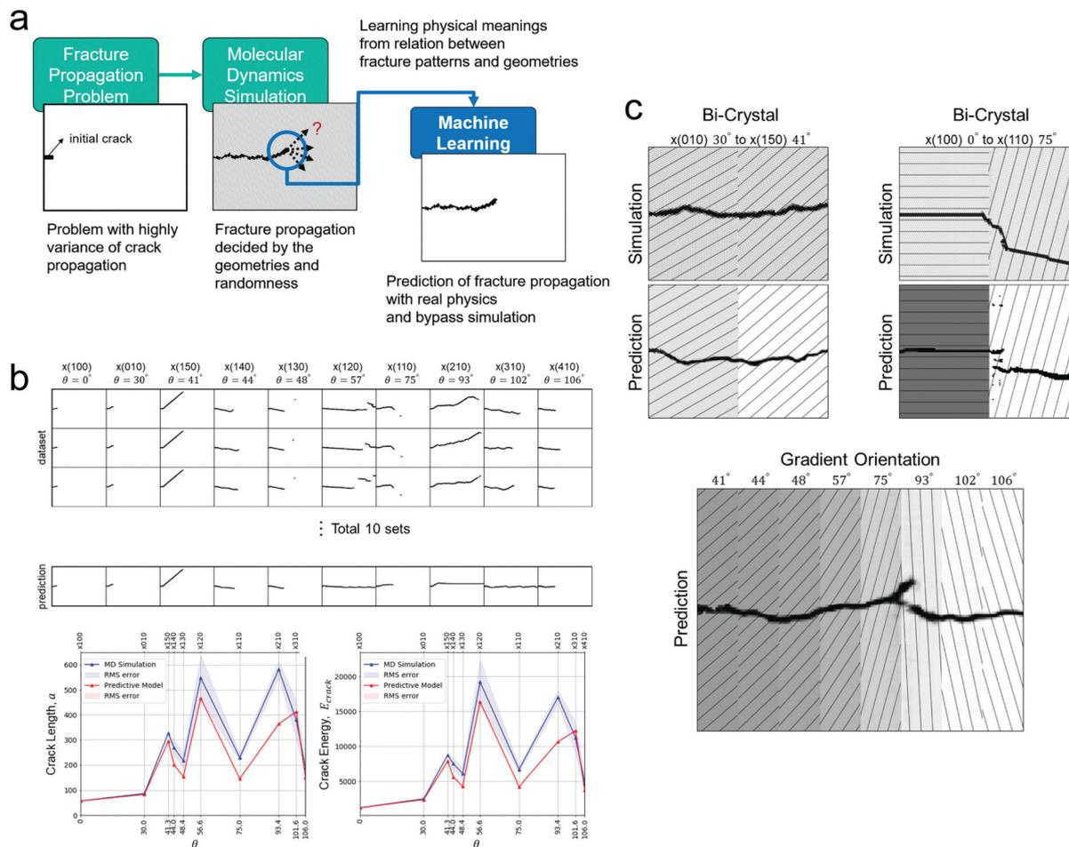
Fig. 4 Predicting dynamical fracture using a deep learning approach, dependent on microstructural details. (a) Workflow of fracture patterns prediction. (b) Comparison of crack path, length and energy release between molecular simulations and the ML approach. (c) Prediction of crack patterns in bicrystalline and gradient materials (Reproduced with permission.<sup>114</sup> Copyright 2020 Elsevier).
