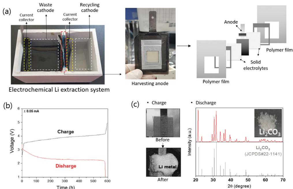
Fig. 10 (a) Prismatic design of electrochemical Li-extraction process. (b) Charge and discharge voltage profile during Li-extraction. (c) Li metal formation after charging and  $\text{Li}_2\text{CO}_3$  formation after discharging.
