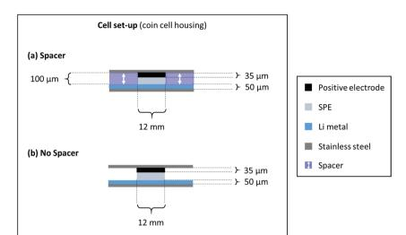
Scheme 1 Cell assembly and respective dimensions of a cell build with (a) spacer and (b) without a spacer.
