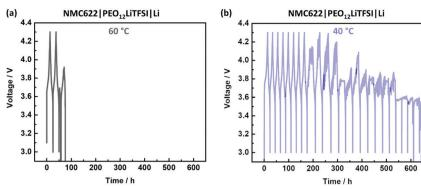
Fig. 1 Charge/discharge cycling of NMC622||Li cells with PEO-based SPE within a voltage range of 4.3-3.0 V and a specific current of 15 mA  $g^{-1}$  ( $\approx 0.1$ C) at (a) 60 °C and (b) 40 °C. The noisy voltage response during charge points to short circuits, whereby the onset of this failure tends to postpone at 40 °C.
