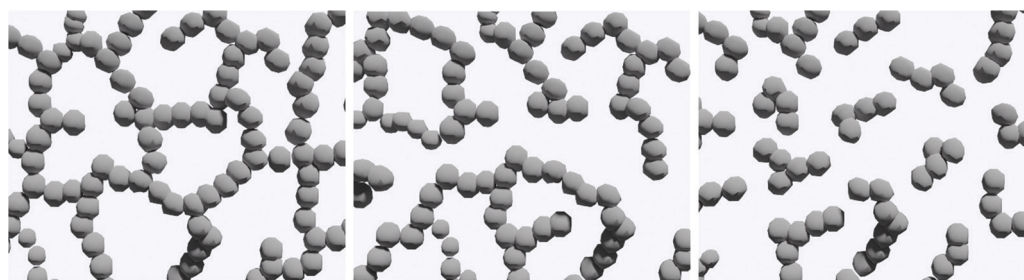
Fig. 5 Microstructure evolution inside a colloidal gel made of a percolated particle network at increasing level of stress.
