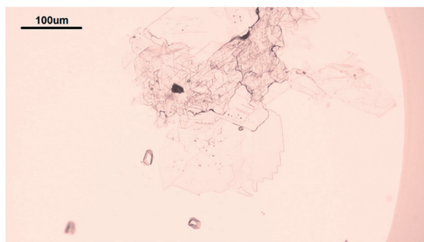
Fig. 6 Insulin crystals (middle towards bottom) in the presence of leucine crystals (top middle part), obtained after 72 days. Leucine forms crystals with sheet like shapes whereas insulin shows rhombohedral shapes.
