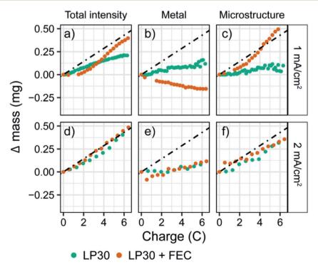
Fig. 3 The fitted intensities of the *in situ* NMR spectra of Li metal for constant currents of (a–c) 1 mA cm<sup>-2</sup> and (d–f) 2 mA cm<sup>-2</sup> in the two electrolytes LP30 (green) and LP30 + FEC (orange). The dashed line indicates  $m_{\text{echem}}$ , the calculated mass deposited according to the current passed by the electrochemistry.
