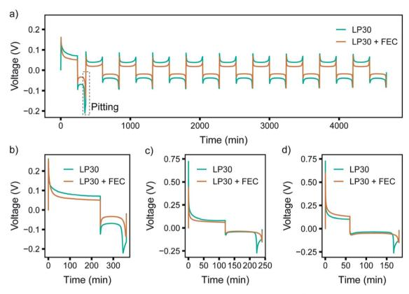
Fig. 4 Galvanostatic cycling of symmetric Li-coin cells during (a) the first 10 cycles at 0.5 mA cm<sup>-2</sup> for both stripping and plating. In the first cycle, shown in the enlargement in (b), 0.5 mA cm<sup>-2</sup> was used for plating and 1.0 mA cm<sup>-2</sup> for stripping. First cycle using (c) 1.0 and (d) 2.0 mA  $cm^{-2}$  plating and 1.0 mA  $cm^{-2}$  for stripping. LP30 (green) and LP30 + FEC (orange). The full cycling data for 1 and 2 mA  $cm^{-2}$  can be found in Fig. S3-S4.†
