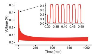
Fig. 5 Representative pulsed current plot for a symmetric Li *in situ* cell at 1 mA cm $^{-2}$  with  $T_{\rm ON}, T_{\rm OFF}=1$  s in the LP30 + FEC electrolyte, also shown in Fig. S26.†
