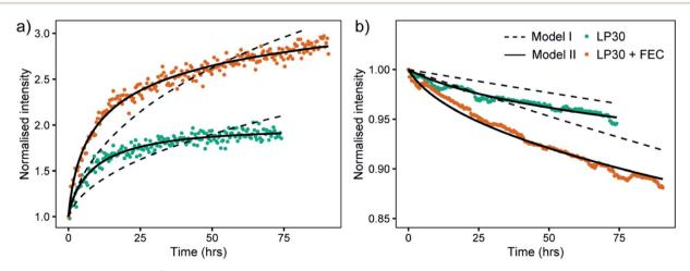
Fig. 9 The intensity changes of the <sup>7</sup>Li NMR spectra (points) and the model fit results for Model I (dashed lines) and Model II (black lines) for (a) the lithium metal and (b) the lithium ions, in the two electrolytes LP30 (green) and LP30 + FEC (orange).
