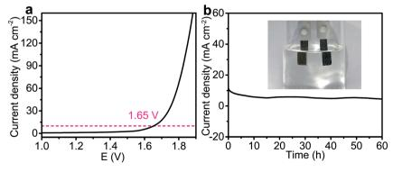
Fig. 5 (a) Performance of the full water-splitting device using the CoFe LDH as the anode and V-Ce/CoFe LDH as the cathode; (b) chronoamperometric curve of CoFe LDH  $\parallel$ V-Ce/CoFe LDH for full water splitting with an overpotential of 10 mA cm $^{-2}$  for 60 h. The inset of b shows the optical photograph of generation gases.
