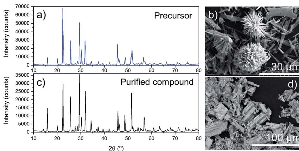
Fig. 4 (a) XRD of precursor and calcined and purified Ta compounds, (b) K<sub>6</sub>Ta<sub>10.8</sub>O<sub>30</sub> particles observed by SEM, (c) SEM image of precursor and (d) K<sub>6</sub>Ta<sub>10.8</sub>O<sub>30</sub> particles observed by SEM.
