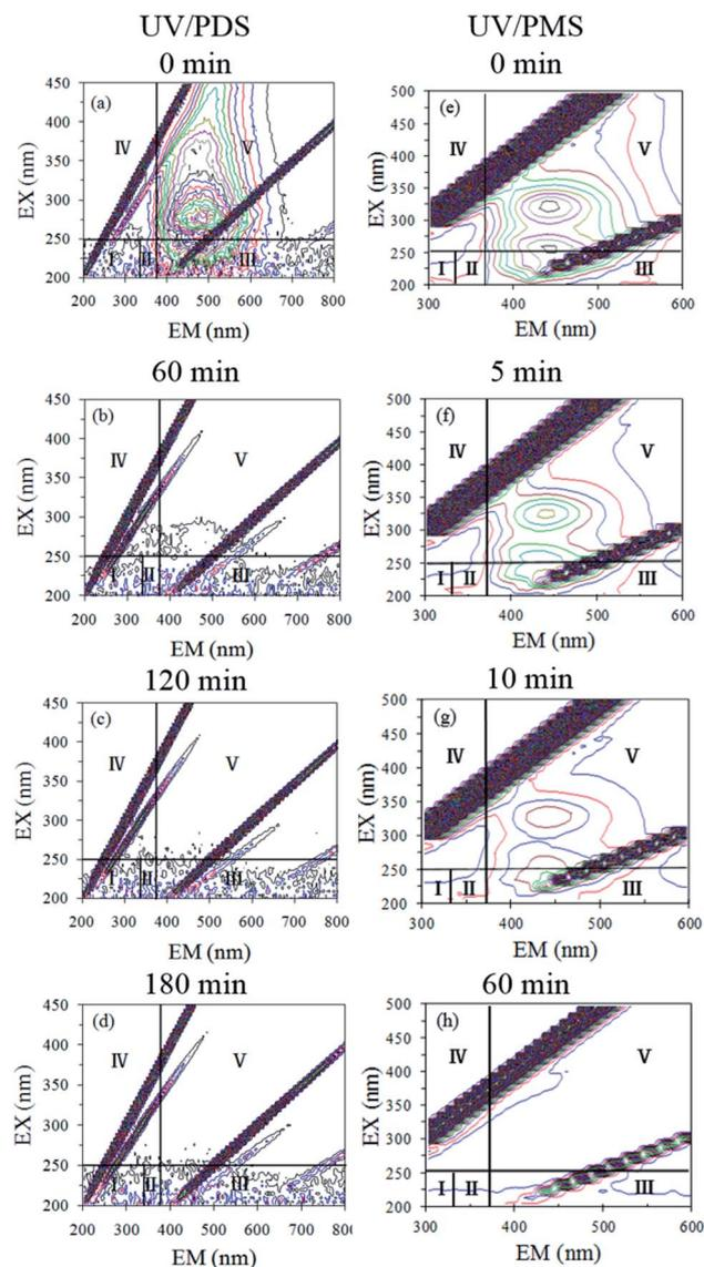
Fig. 6 3D-EEM spectra of HA at various reaction times in UV/PDS (a–d) and UV/PMS (e–h). Conditions:  $[HA]_0 = 15 \text{ mg L}^{-1}$ ,  $[PDS]_0 = 3 \text{ mmol L}^{-1}$ ,  $[PMS]_0 = 1 \text{ mmol L}^{-1}$ ,  $\text{pH}_0 = 6$  and  $3$  for UV/PDS and UV/PMS, respectively.
