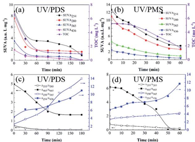
Fig. 5 Evolution of the SUVA and UV spectroscopic ratios during HA removal in UV/PDS (a and c) and UV/PMS (b and d). Conditions:  $[HA]_0 = 15 \text{ mg L}^{-1}$ ,  $[PDS]_0 = 3 \text{ mmol L}^{-1}$ ,  $[PMS]_0 = 1 \text{ mmol L}^{-1}$ ,  $\text{pH}_0 = 6$  and  $3$  for UV/PDS and UV/PMS, respectively.
