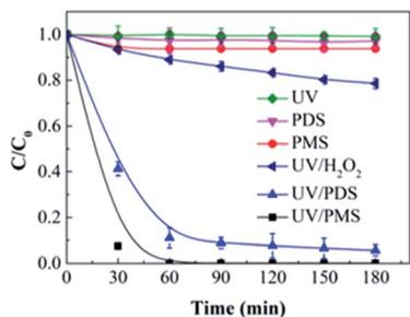
Fig. 1 HA elimination with the UV, PDS, PMS, UV/PDS, UV/PMS, and UV/H<sub>2</sub>O<sub>2</sub> processes. Conditions: [HA]<sub>0</sub> = 15 mg L<sup>-1</sup>, [PDS]<sub>0</sub> = [PMS]<sub>0</sub> = [H<sub>2</sub>O<sub>2</sub>]<sub>0</sub> = 3 mmol L<sup>-1</sup>, pH<sub>0</sub> = 6, 3, and 4 for UV/PDS, UV/PMS, and UV/H<sub>2</sub>O<sub>2</sub>, respectively.
