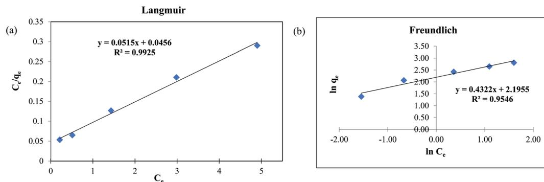
Fig. 5 Adsorption isotherm of MOF-801 as (a) Langmuir and (b) Freundlich isotherms for fluoride adsorption. Test conditions: adsorbent (1 g L<sup>-1</sup>), reaction time (120 min) and fluoride solution (20 mL).
