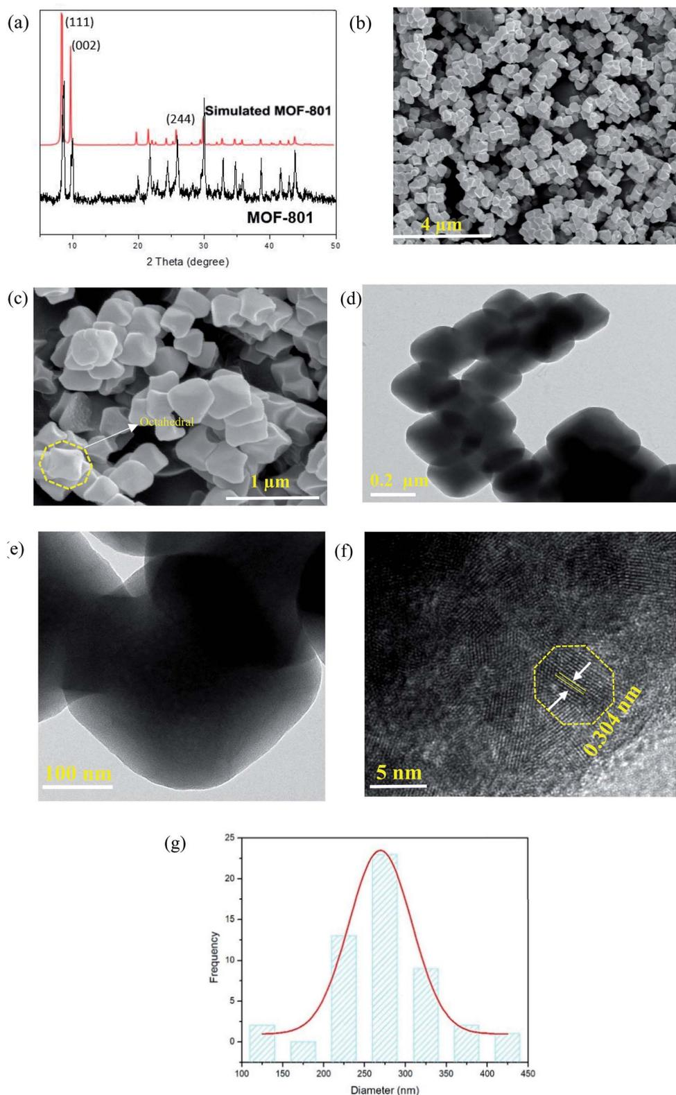
Fig. 2 (a) PXRD of MOF-801, FESEM of MOF-801 at (b) low magnification (25k $\times$ ); (c) high magnification (100k $\times$ ), TEM of MOF-801 at (d) low magnification (2.3k $\times$ ); (e) high magnification (8.9k $\times$ ), (f) HRTEM of MOF 801 and (g) particle size distribution of MOF-801.
