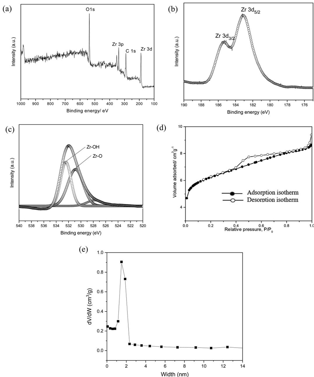
Fig. 3 (a) XPS wide scan of MOF-801, narrow scan of (b) Zr 3d, (c) O 1s, (d) the adsorption–desorption isotherm of N<sub>2</sub> in MOF-801 at 77 K and (e) pore size distribution of MOF-801.
