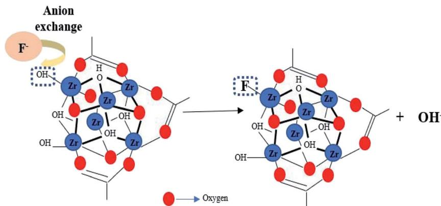
Fig. 7 Proposed mechanism of MOF-801 for fluoride adsorption.
