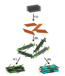
Fig. 14 Schematic illustration of aqueous dispersions of (A) GO, (B) GO-PDI and (C) GO-PyS through  $\pi-\pi$  interaction and (D) coassembly of negatively charged ssDNA-G sheets and positively charged cytochrome c produces co-intercalated multifunctional layered nanocomposites. This figure has been reproduced from ref. 93 with permission from *Adv. Mater.*, Copyright 2009.
