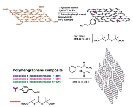
Fig. 10 Preparation of polymer-graphene composites. This figure has been reproduced from ref. 81 with permission from *J. Colloid Interface Sci.*, Copyright 2017.
