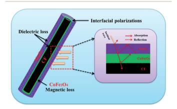
Fig. 10 Mechanism illustration of microwave absorption for the  $CF@CoFe_2O_4@MnO_2$  composite.
