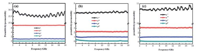
Fig. 7 Electromagnetic parameters of CF (a), CF@CoFe<sub>2</sub>O<sub>4</sub> (b) and CF@CoFe<sub>2</sub>O<sub>4</sub>@MnO<sub>2</sub> composite (c).
