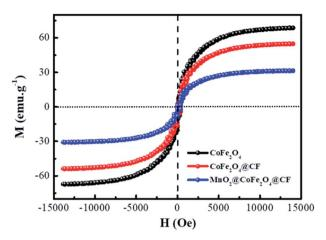
Fig. 6 Hysteresis loops of  $CoFe_2O_4$ ,  $CF@CoFe_2O_4$  and  $CF@CoFe_2-O_4@MnO_2$  composites.
