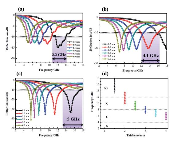
Fig. 9 Reflection loss curves of CF (a),  $CF@CoFe_2O_4$  (b) and  $CF@CoFe_2O_4@MnO_2$  composites (c) at a different thickness, the effective absorption band width of  $CF@CoFe_2O_4@MnO_2$  composite (d).
