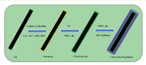
Fig. 1 Explanation of the preparation process of the CF@CoFe<sub>2</sub>O<sub>4</sub>@MnO<sub>2</sub> composite.
