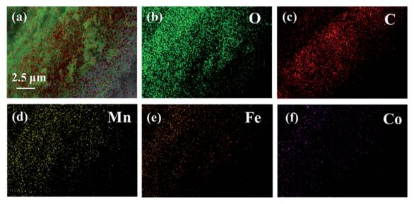
Fig. 3 EDX elemental mapping images (a-f) of CF@CoFe<sub>2</sub>O<sub>4</sub>@MnO<sub>2</sub> composite.
