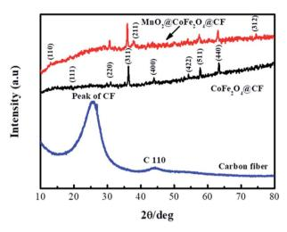
Fig. 4 XRD patterns of CF, CF@CoFe $_2$ O $_4$  and CF@CoFe $_2$ O $_4$ @MnO $_2$  composites.
