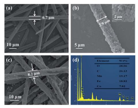
Fig. 2 SEM images of CF (a), CF@CoFe $_2$ O $_4$ @MnO $_2$  composites (c) and the EDS spectra of CF@CoFe $_2$ O $_4$ @MnO $_2$  composite (d).
