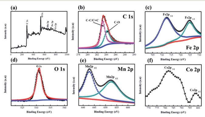
Fig. 5 XPS spectra of CF@CoFe<sub>2</sub>O<sub>4</sub>@MnO<sub>2</sub> composite, a survey scan (a), C 1s (b), Fe 2p (c), O 1s (d), Mn 2p (e), Co 2p (f).
