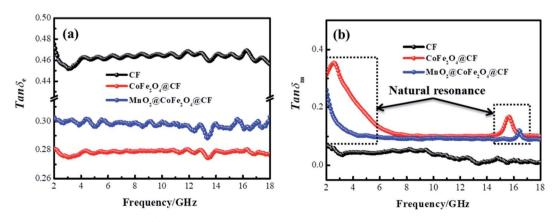
Fig. 8 Dielectric loss (a) and magnetic loss (b) of CF,  $CF@CoFe_2O_4$  and  $CF@CoFe_2O_4@MnO_2$  composites.
