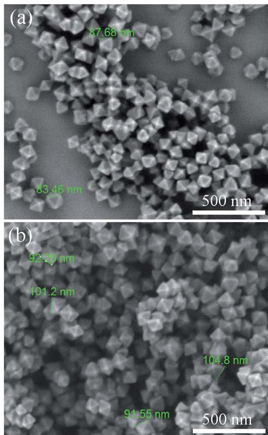
Fig. 2 FE-SEM images of (a) UiO-66-NH<sub>2</sub> and (b) UiO-66-NH<sub>2</sub>-PC.
