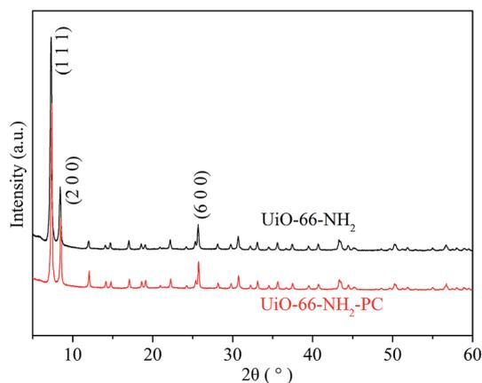
Fig. 3 XRD patterns of UiO-66-NH<sub>2</sub> and UiO-66-NH<sub>2</sub>-PC.
