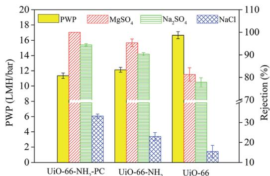
Fig. 17 Nanofiltration performance of TFN membranes prepared with different MOF nanomaterials.
