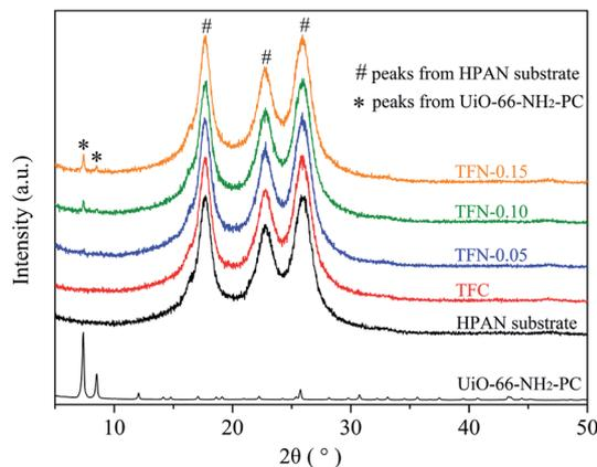
Fig. 10 XRD patterns of UiO-66-NH<sub>2</sub>-PC, HPAN substrate and the prepared membranes.
