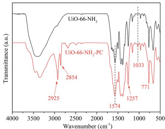
Fig. 4 FT-IR spectra of UiO-66-NH<sub>2</sub> and UiO-66-NH<sub>2</sub>-PC.
