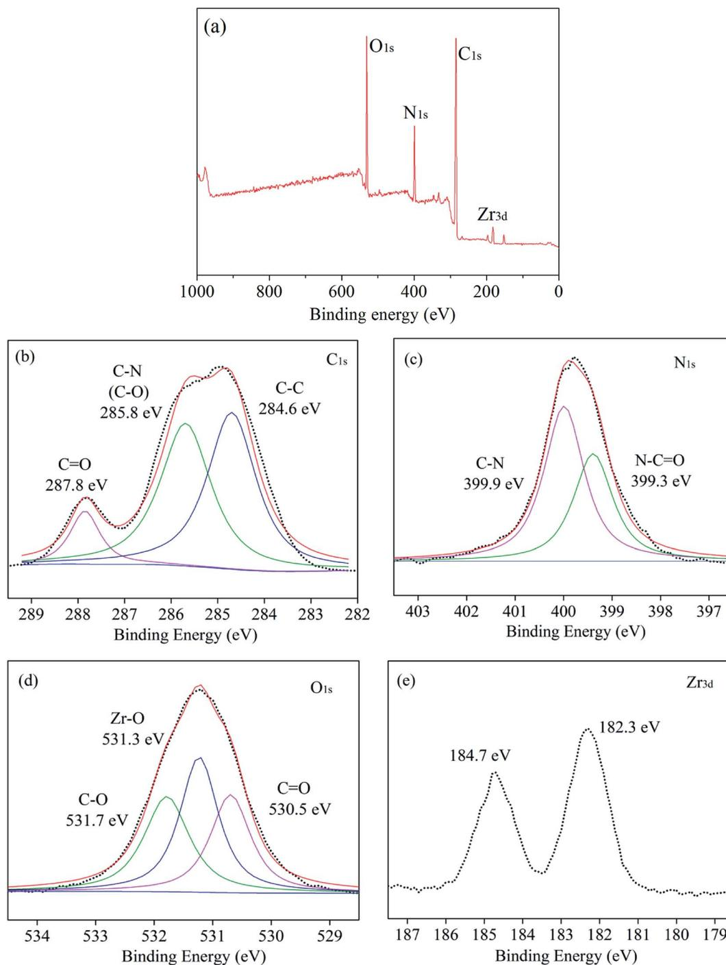
Fig. 9 XPS survey spectra of TFN-0.10 membrane.
