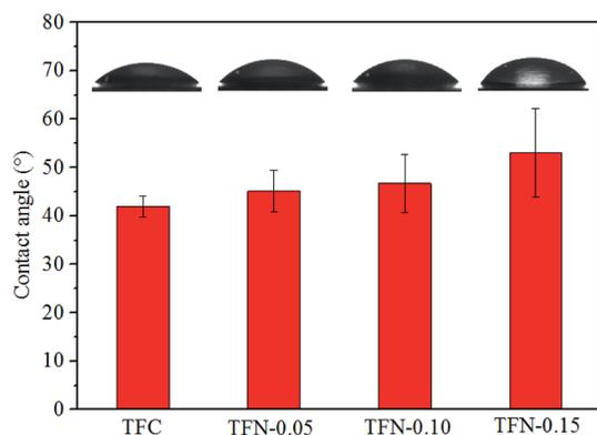
Fig. 11 Contact angle of TFC and TFN membranes.
