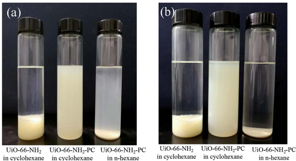
Fig. 5 Dispersibility of UiO-66-NH<sub>2</sub> and UiO-66-NH<sub>2</sub>-PC in cyclohexane and *n*-hexane after standing for (a) 30 min and (b) 12 h.
