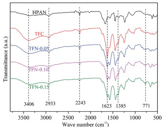
Fig. 8 ATR-FTIR spectra of the prepared membranes.
