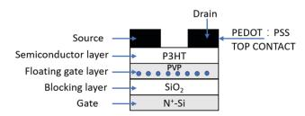
Fig. 1 Schematic of a top contact floating gate OFET memory device.
