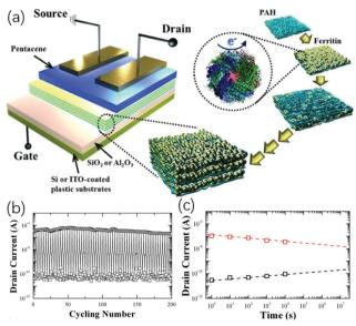
Fig. 3 (a) Schematic representation of the OFET memory device with LBL-assembled (PAH/ferritin NP) $_n$  multi-layered gate dielectrics. (b) Cycling and (c) retention time tests for devices with (PAH/ferritin NP)<sub>40</sub> multi-layers. Reproduced with permission.<sup>37</sup> Copyright 2013, John Wiley and Sons.
