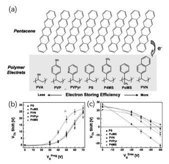
Fig. 6 (a) Schematic representation of the electron-storage efficiency of polymer electret materials estimated from the PEM characteristics. Shifts in V<sub>th</sub> of PEM devices after the application of different gate biases during the (b) programming and (c) erasing processes. The dotted lines are fits to the measured points using a sigmoid function (Boltzmann fits). Reproduced with permission. 51 Copyright 2008, John Wiley and Sons.
