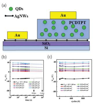
Fig. 16 (a) Schematic illustration of the photonic memory transistor. The retention curves of  $V_{\rm th}$  (b) and the endurance curves of  $V_{\rm th}$  (c) of photonic memory devices after light programming under light illumination (300 nm) with different light intensities for 0.5 s and after electric erasing with gate bias  $V_G = -10 \text{ V}$  for 100 ms. Reproduced with permission.<sup>79</sup> Copyright 2020, Royal Society of Chemistry
