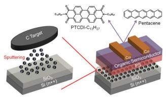
Fig. 4 Schematic representation of a pentacene-based or PTCDI-C<sub>13</sub>H<sub>27</sub>-based floating gate OFET memory device (right), in which a PS layer and sputtered C-NPs (left) on top are employed as a tunnelling dielectric and nano floating gate, respectively. Reproduced with permission.<sup>41</sup> Copyright 2014, AIP Publishing.
