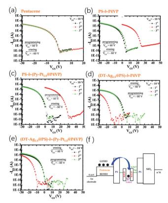
Fig. 10  $V_{th}$  shifts in the transfer characteristics of the devices incorporating (a) bare SiO<sub>2</sub>, (b) PS-b-P4VP, (c) PS-b-(Py-Pt1.0@P4VP), (d) (DT-Ag1.0@PS)b-P4VP, and (e) (DT-Ag1.0@PS)-b-(PyPt1.0@P4VP). (f) Schematic diagram of the carrier tunnelling through the polymer electret into the metal NPs. Reproduced with permission.<sup>57</sup> Copyright 2013, Royal Society of Chemistry.
