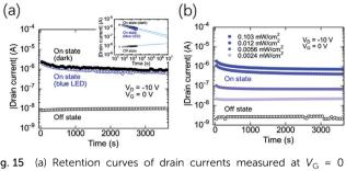
Fig. 15 (a) Retention curves of drain currents measured at  $V_G = 0$  V and  $V_D = -10 \text{ V}$  in the dark and under blue light illumination (469 nm, 1.06 mW cm<sup>-2</sup>) before and after programming with blue light. (b) Retention curves measured in the dark before and after programming ( $V_G$  = +60 V, 3 s) with blue light at different intensities. Reproduced with permission.90 Copyright 2019, Elsevier.
