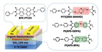
Fig. 7 Schematic diagram of the studied polymer electret OFET memory devices and the molecular structures of the studied PIs. Reproduced with permission.<sup>55</sup> Copyright 2014, John Wiley and Sons.
