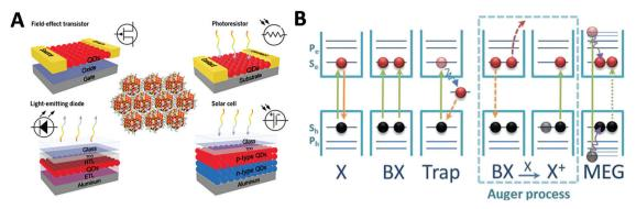
Fig. 8 Schematic representation of various devices using TQDs (A) and the spectroscopic understanding of charge separation and recombination processes involving trapping, particle charging, Auger recombination, and MEG that are crucial in the devices (B). X: exciton, BX: biexciton, MEG: multiple exciton generation. Adapted with permission from ref. 9, copyright 2016, the American Association for the Advancement of Science.
