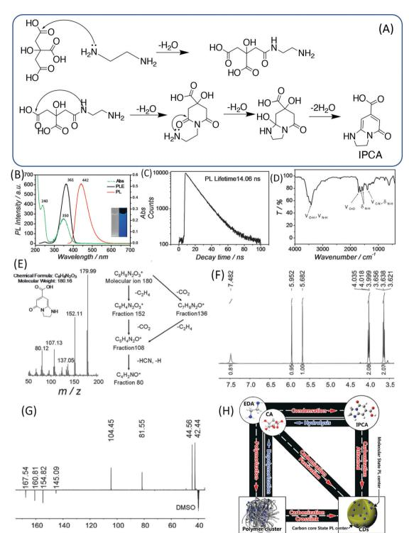
Fig. 4 (A) The assumed process of forming the molecule (IPCA) from CA and EDA. (B) UV-vis absorption, PL emission and excitation spectra of IPCA; inset: photographs of IPCA solution under visible and UV light. (C) Time-resolved PL lifetime decay, (D) FTIR, (E) mass spectrum, (F) <sup>1</sup>H NMR, and (G) DEPTQ <sup>13</sup>C NMR spectra of IPCA. (H) A schematic of the relationship between different products in the one-pot hydrothermal system of CA and EDA.<sup>24</sup>
