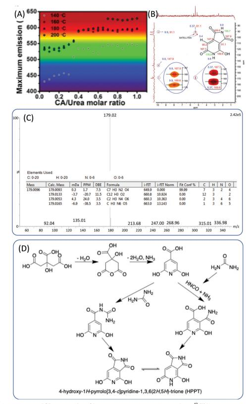
Fig. 7 (A) The maximum emission of CDs prepared from CA and urea under various reaction conditions.<sup>49</sup> (B) Heteronuclear multiple bond coherence (HMBC) <sup>1</sup>H-<sup>13</sup>C NMR spectrum of HPPT and chemical structure of HPPT with NMR assignments (ppm). (C) High-resolution mass spectrum of HPPT showing a molecular ion peak with m/z (ESI-) = 179, and indicating the molecular formula  $C_7H_4N_2O_4$ . (D) Possible mechanism of HPPT formation.<sup>55</sup>
