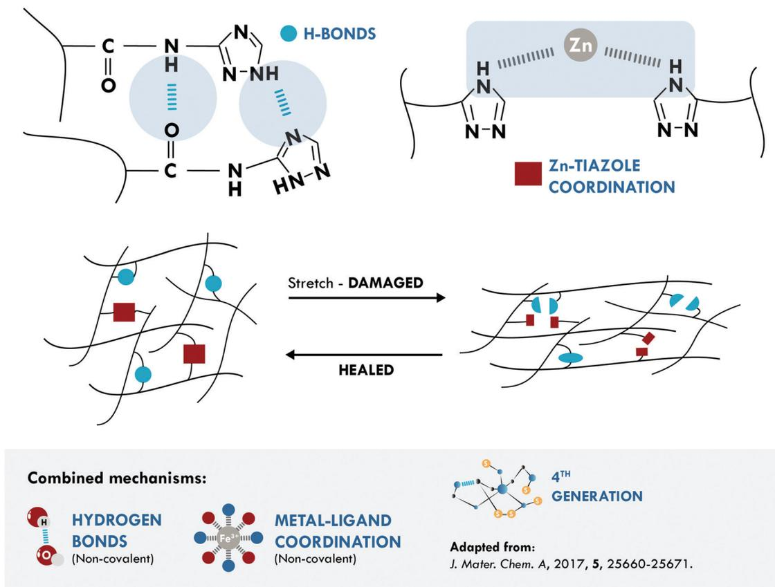
Fig. 7 Combination between hydrogen bonds and metal–ligand coordination in IR.<sup>172</sup> ©2017. Adapted with permission from the Royal Society of Chemistry.
