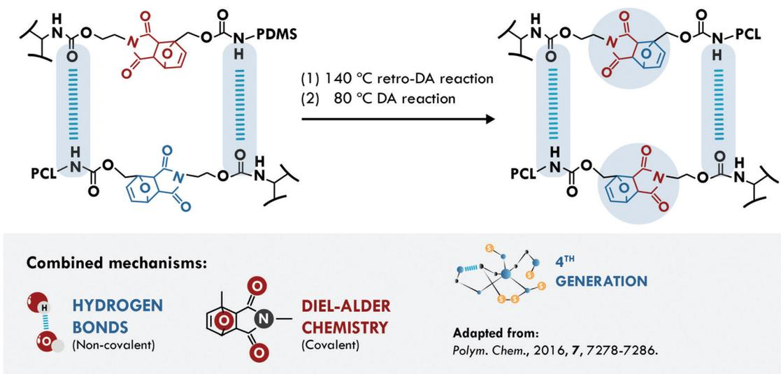
Fig. 11 Combination between DA chemistry and hydrogen bonds in PDMS-DA-PU.<sup>200</sup> ©2016. Adapted with permission from the Royal Society of Chemistry.
