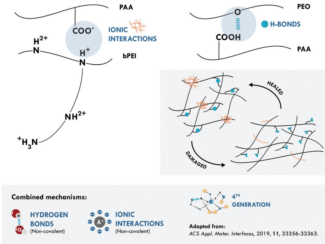
Fig. 6 Combination between hydrogen bonds and ionic interactions in bPEI/PAA/PEO.<sup>167</sup> ©2019. Adapted with permission from the American Chemical Society.
