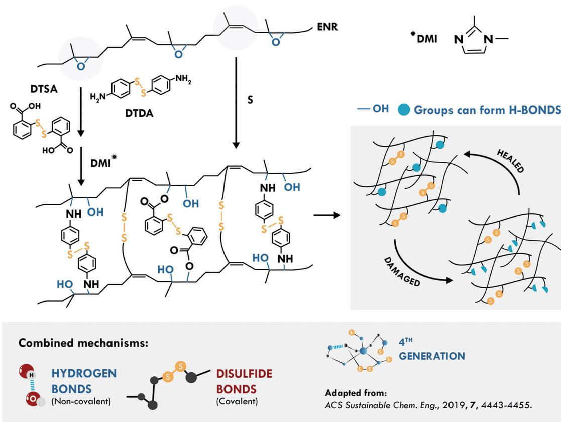
Fig. 10 Combination between disulfide and hydrogen bonds in ENR.<sup>194</sup> ©2019. Adapted with permission from the American Chemical Society.
