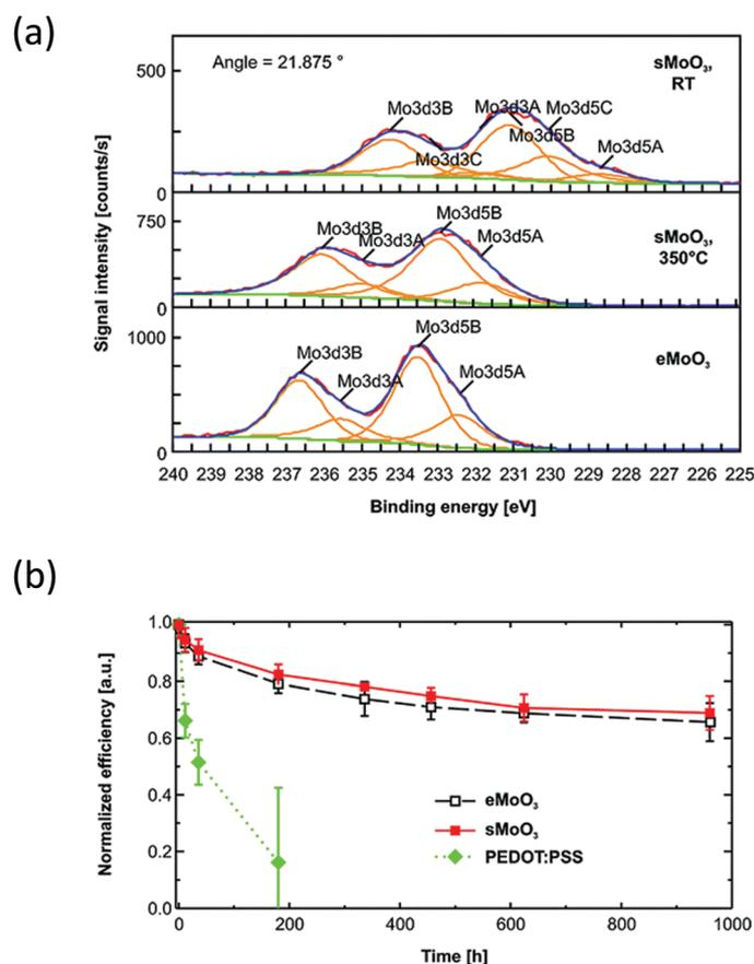
Fig. 8 (a) X-Ray photoelectron spectroscopy of solution-processed MoO<sub>3</sub> (sMoO<sub>3</sub>) compared to an evaporated film (eMoO<sub>3</sub>) and (b) stability of OPV devices with P3HT:PC<sub>61</sub>BM active layer, stored in ambient conditions reported by Rand *et al.*<sup>60</sup> Reprinted with permission from ref. 60. Copyright 2011 American Chemical Society.
