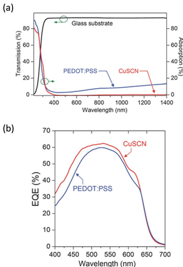
Fig. 9 (a) Transmittance of CuSCN compared to PEDOT:PSS (top), and (b) EQE plots for P3HT:ICBA-based OPV devices containing the two hole transport layers.<sup>72</sup> Reproduced with permission.<sup>72</sup> Copyright 2015, WILEY-VCH Verlag GmbH & Co. KGaA, Weinheim.
