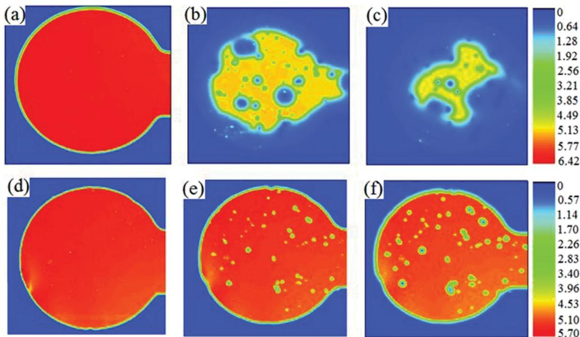
Fig. 5 Laser beam induced photocurrent images of the devices exposed to ambient air: (a and d) 0 days; (b and e) 4 days and (c and f) 8 days. The hole-transport layer was PEDOT:PSS (a–c) or MoO<sub>3</sub>-PEDOT:PSS (d–f). The colour scale represents the photocurrent. Reproduced with permission.<sup>41</sup> Copyright 2013, WILEY-VCH Verlag GmbH & Co. KGaA, Weinheim.
