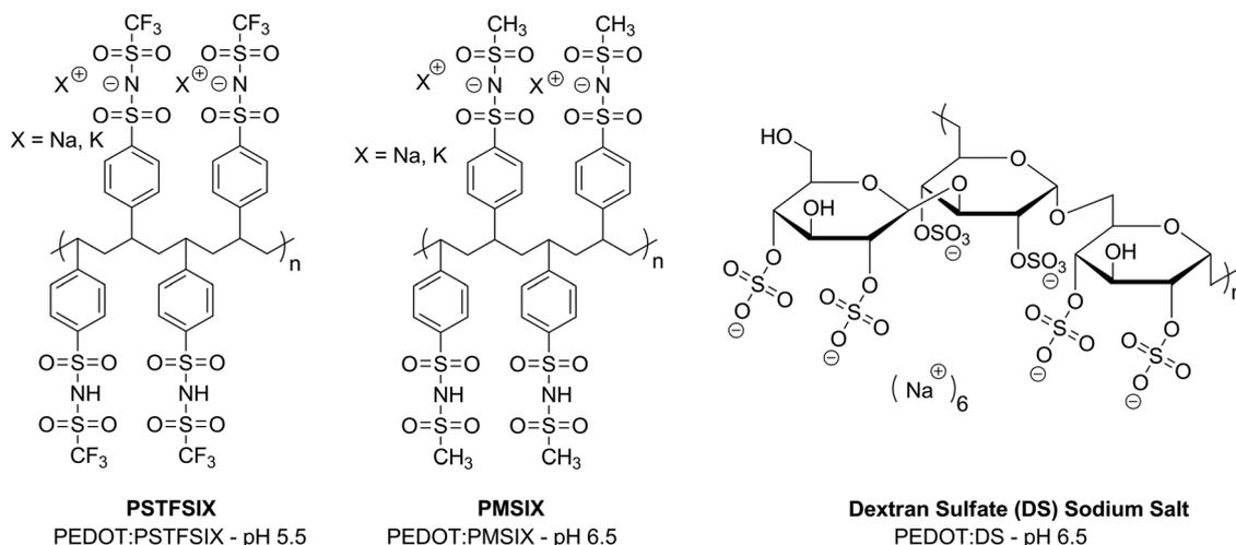
Fig. 6 Examples of polyelectrolytes that have been used with PEDOT complexes, reported by Hadziioannou *et al.*<sup>46</sup>
