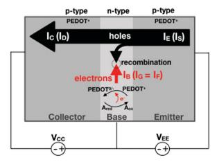
**Fig. 4** Conceptual structure of a bipolar-junction-transistor based on a PEDOT:PSS OECT serving as an amperometric sensor to detect and amplify the faradaic current generated by the species A undergoing an oxidation process in the base region.
