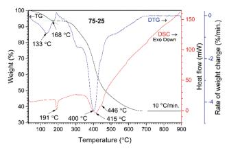
Fig. 4 TG/DTG and DSC curves of acrylate(75%)-gelatin(25%)-cHAP
