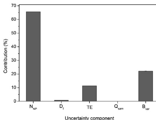
**Fig. 3** Typical uncertainty budget for dynamic mass flow method, using 30 nm Au NP as an example.  $N_{\text{NP}}$  is the number of particles detected in time scan,  $D_f$  is sample dilution factor, TE is the transport efficiency,  $Q_{\text{sam}}$  is the sample mass flow and  $B_{\text{var}}$  is the batch-to-batch variability.
