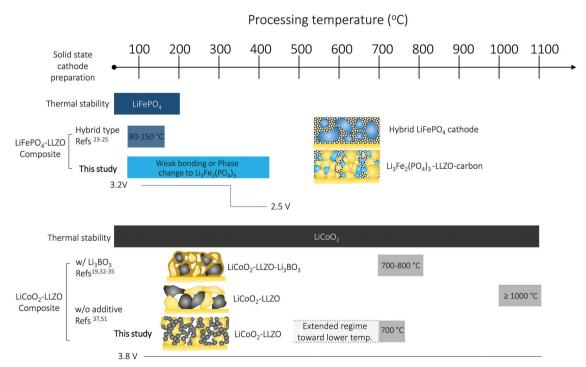
Fig. 6 Overview of the cathode composite design and ceramic processing choices of all-oxide Li-garnet SSBs based on LiFePO<sub>4</sub>- and LiCoO<sub>2</sub>-based cathode composites: processing temperature vs. chemical and mechanical stability
