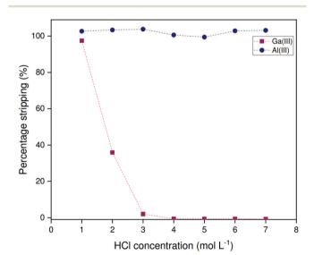
Fig. 8 Percentage stripping of gallium and aluminum as a function of the HCl concentration in the stripping liquor for loaded 5 vol% Kelex® 100 in [HHT<sub>12</sub>][Tf<sub>2</sub>N] modified with 10 vol% 1-decanol, extracted from 200 ppm solutions containing 2.000 mol  $L^{-1}$  sodium hydroxide in 1:1 phase ratio (organic to aqueous). Temperature: 22 °C.
