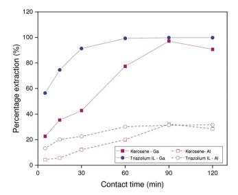
Fig. 6 Percentage extraction as a function of time for 200 ppm solutions extracted from 1.700 mol L $^{-1}$  sodium carbonate by 5 vol% Kelex® 100 in [HHT $_{12}$ ][Tf $_2$ N] modified with 10 vol% 1-decanol, and 5 vol% Kelex® 100 in kerosene modified with 10 vol% 1-decanol. Phase ratio: 1:1 organic to aqueous. Temperature: 22 °C.
