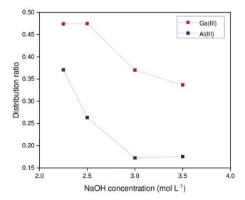
Fig. 9 Distribution ratio of gallium as a function of the NaOH concentration in the stripping liquor for loaded 0.124 mol mol $^{-1}$  Kelex $^{\odot}$  100 in [EhEhT $_{23}$ ] $_4$ [SO $_4$ ], extracted from 200 ppm solutions containing 1.700 mol L $^{-1}$  sodium carbonate in 1:1 phase ratio (organic to aqueous). Temperature: 22 °C.
