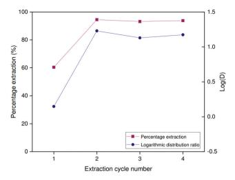
Fig. 10 Percentage extraction and logarithmic distribution ratio of gallium over several extraction/stripping cycles. Extraction was performed in 1:1 phase ratio by 5 vol% Kelex 100 in [HHT<sub>12</sub>][Tf<sub>2</sub>N] (modified with 10 vol% 1-decanol) from 2 mol L $^{-1}$  NaOH containing 873 mmol L $^{-1}$  NaAl(OH) $_4$  and 150 ppm Ga. Stripping was performed with 1 mol L $^{-1}$  HCl. Temperature: 22 °C.
