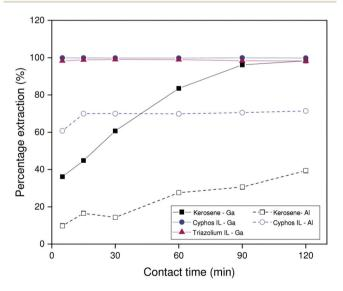
Fig. 5 Percentage extraction as a function of time for 200 ppm solutions extracted from 1.700 mol L $^{-1}$  sodium carbonate by 5 vol% Kelex® 100 in [EhEhT $_{23}$ ]<sub>2</sub>[SO<sub>4</sub>], 5 vol% Kelex® 100 in [C101]<sub>2</sub>[SO<sub>4</sub>] and 5 vol% Kelex® 100 in kerosene modified with 10 vol% 1-decanol. Phase ratio: 1:1 organic to aqueous. The HLLE procedure was followed for [EhEhT $_{23}$ ]<sub>2</sub>[SO<sub>4</sub>].
