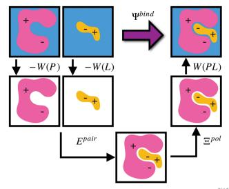
Fig. 1 Schematic illustrating the decomposition of binding energy,  $\Psi^{\text{bind}}$ , into desolvation free energy of the protein, -W(P), the desolvation free energy of the ligand, -W(L), the intermolecular pairwise interaction energy,  $E^{\text{pair}}$ , the ligand polarization energy,  $\Xi^{\text{pol}}$ , and the solvation free energy of the complex, W(PL).
