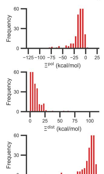
**Fig. 2** Histograms of the ligand polarization (top,  $\mathcal{Z}^{\text{pol}}$ ), distortion (middle,  $\mathcal{Z}^{\text{dist}}$ ), and stabilization (bottom,  $\mathcal{Z}^{\text{stab}}$ ) energies in the PDBBind Core Set. The three quantities are related by  $\mathcal{Z}^{\text{pol}} = \mathcal{Z}^{\text{dist}} + \mathcal{Z}^{\text{stab}}$ .
