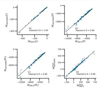
Fig. 10 Comparison of solvation free energy estimates (in kcal  $mol^{-1}$ ) based on OBC2 (x-axis) and ddCOSMO (y-axis). Solvation free energy estimates are of the (a) ligand, (b) protein, (c) complex, and (d) the binding
