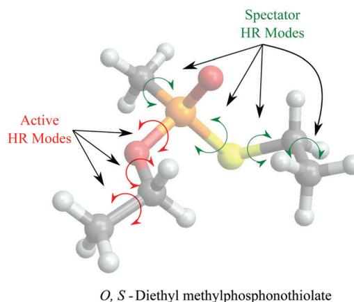
Fig. 3 Illustration of the active and spectator HR modes of *O,S*-diethyl methylphosphonothiolate for the O-side reaction. The curved red arrows indicate the rotations across the single bonds in the active HR modes, the curved green arrows are for the inactive HR modes.
