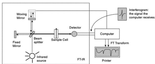
Fig. 1 Schematic diagram by Pavia *et al.*<sup>10</sup> of an FTIR instrument. From Pavia/Lampman/Kriz/Vyvan. Introduction to Spectroscopy, 4E. © 2009 Brooks/Cole, a part of Cengage, Inc. Reproduced by permission. <http://www.cengage.com/permissions>.
