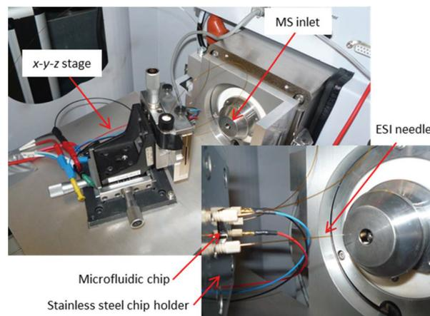
**Fig. 20** Photographs of a microfluidic EC cell integrated with a commercially available ESI needle in an EC-MS setup. Reprinted with permission from van den Brink *et al.*<sup>287</sup> Copyright 2015 American Chemical Society.
