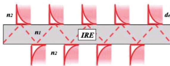
Fig. 4 Internal reflection element. Reprinted and adapted from the original work by Schadle and Mizaikoff,<sup>68</sup> Copyright 2016, with permission from SAGE Publications.
