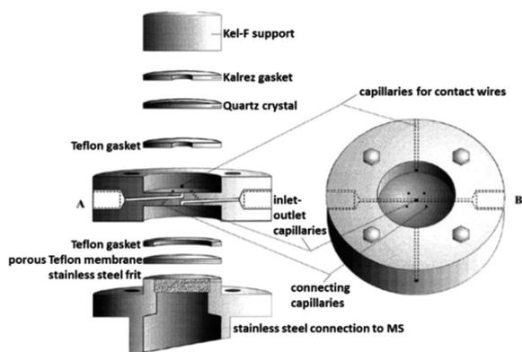
Fig. 23 DEMS cell; A: exploded sideview; B: top view. Image republished and modified with permission of Journal of The Electrochemical Society, from the original work by Jusys *et al.*<sup>297</sup> Copyright 1999, permission conveyed through Copyright Clearance Center, Inc.
