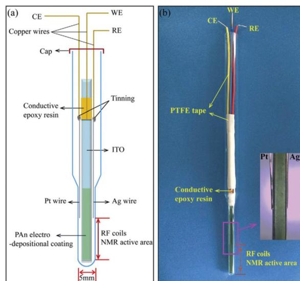
**Fig. 17** Schematic and photograph of an ITO/PAN WE based three-electrode NMR-SEC cell. Reprinted from the original work by Zhang *et al.*,<sup>271</sup> Copyright 2018, with permission from Elsevier.
