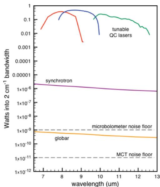
Fig. 7 Comparison of Weida and Yee of three different IR sources of the signal through a 10 μm pinhole.<sup>96</sup> Reprinted and adapted from the original work by Weida and Yee,<sup>96</sup> Copyright 2011, with permission from SPIE and M. Weida.
